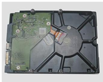
3. Align holes on the disk with holes on the bottom cover.
