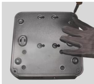
2. Fix the four screws on the disk without fully tightening them.
