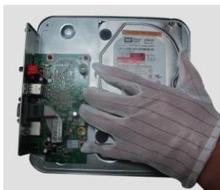
4. Secure the disk to the bottom cover using four screws.
